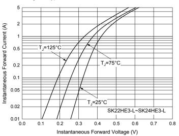
Fig. 5 - Typical Instantaneous Forward Characteristics
