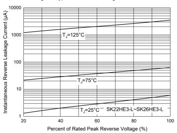
Fig. 8 - Typical Reverse Leakage Characteristics
