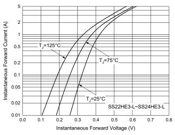
Fig. 5 - Typical Instantaneous Forward Characteristics
