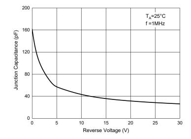
Fig.9 Capacitance Characteristics
