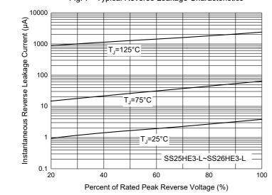
Fig. 7 - Typical Reverse Leakage Characteristics
